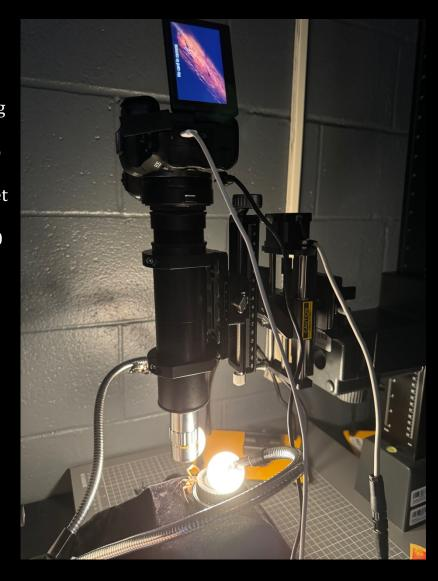
The image on the page shows the setup to capture the 10x image. The subject is set up below the Mitutoyo 10x optics lens system attached to the focus rail on the copy stand. The fiber optic lights are on each side lighting the subject. The other lenses were used for other magnifications.
